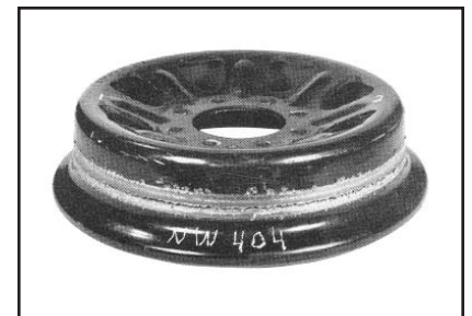
▲ Pressed steel wheel after only 3.5 hours under 5,000 lb. load shows EXTENSIVE wear.
