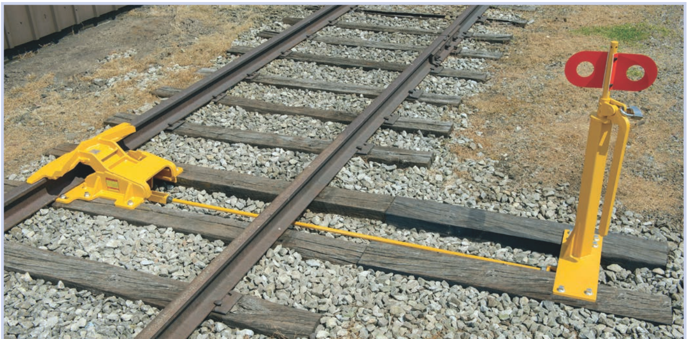
▲ Shown above is a Double-end Sliding Derail with an LSE-2 Standard Operating Stand and Connecting Rod set up in a far rail application. Operating stands and connecting rods are sold separately from derails. All Nolan operating stands can be padlocked. (Padlocks not included.)
