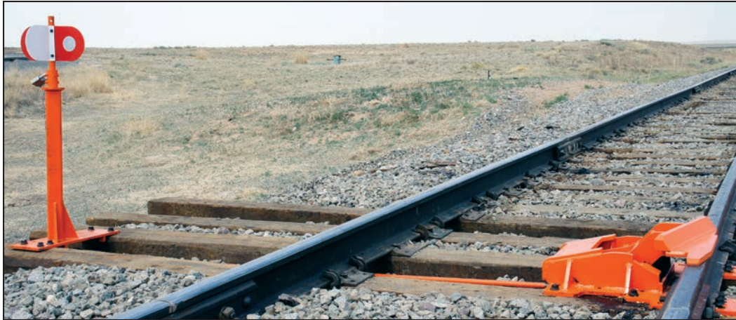
▲ Single-end Sliding Derail with an LSE-2 Standard Operating Stand and Connecting Rod set up in a far rail application. Operating stands and connecting rods are sold separately from derails. All Nolan operating stands can be padlocked. (Padlocks not included.)
