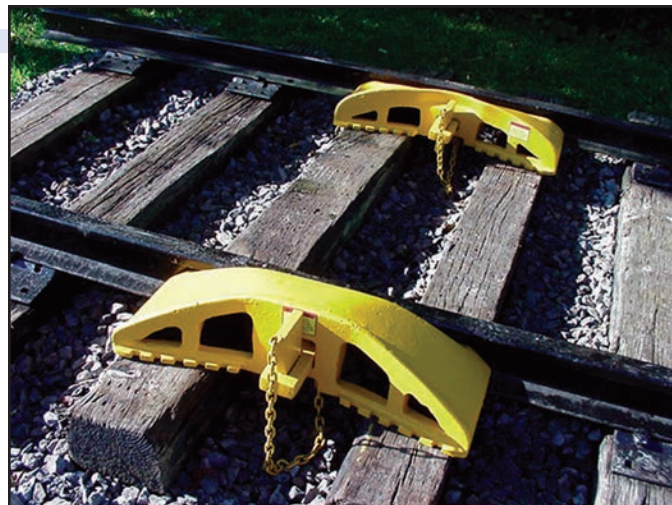
▲ SWA Rerailers (IN and OUT) on the track
