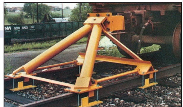
▲ HDBP Bumping Post w/optional Cushion Head (CH)
