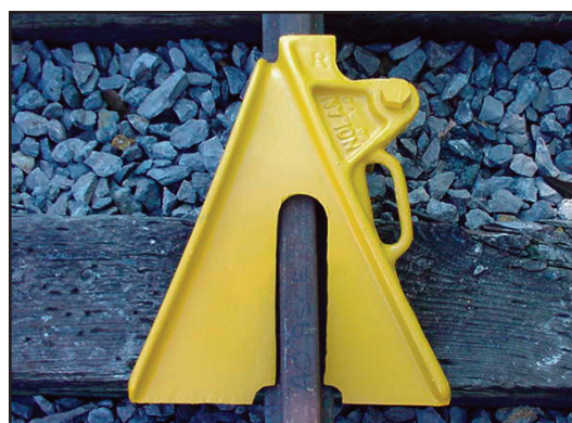
▲ CW-3R Rerailer on the track
