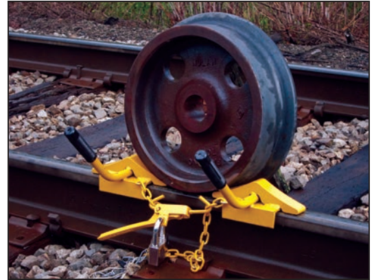
▲ WC-11-101 Wheel Chock shown positioned with wheel
