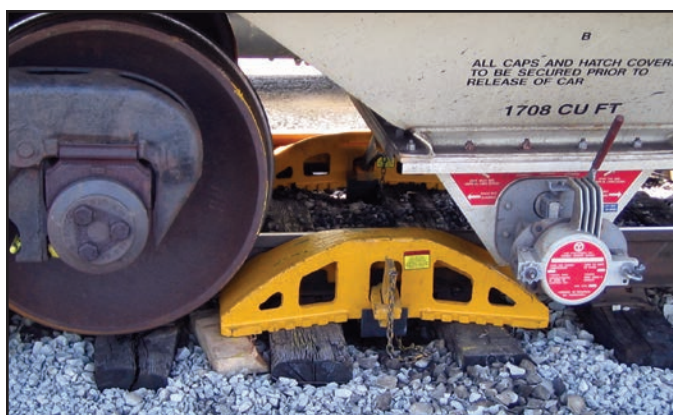
▲ SWB Rerailers on the job
